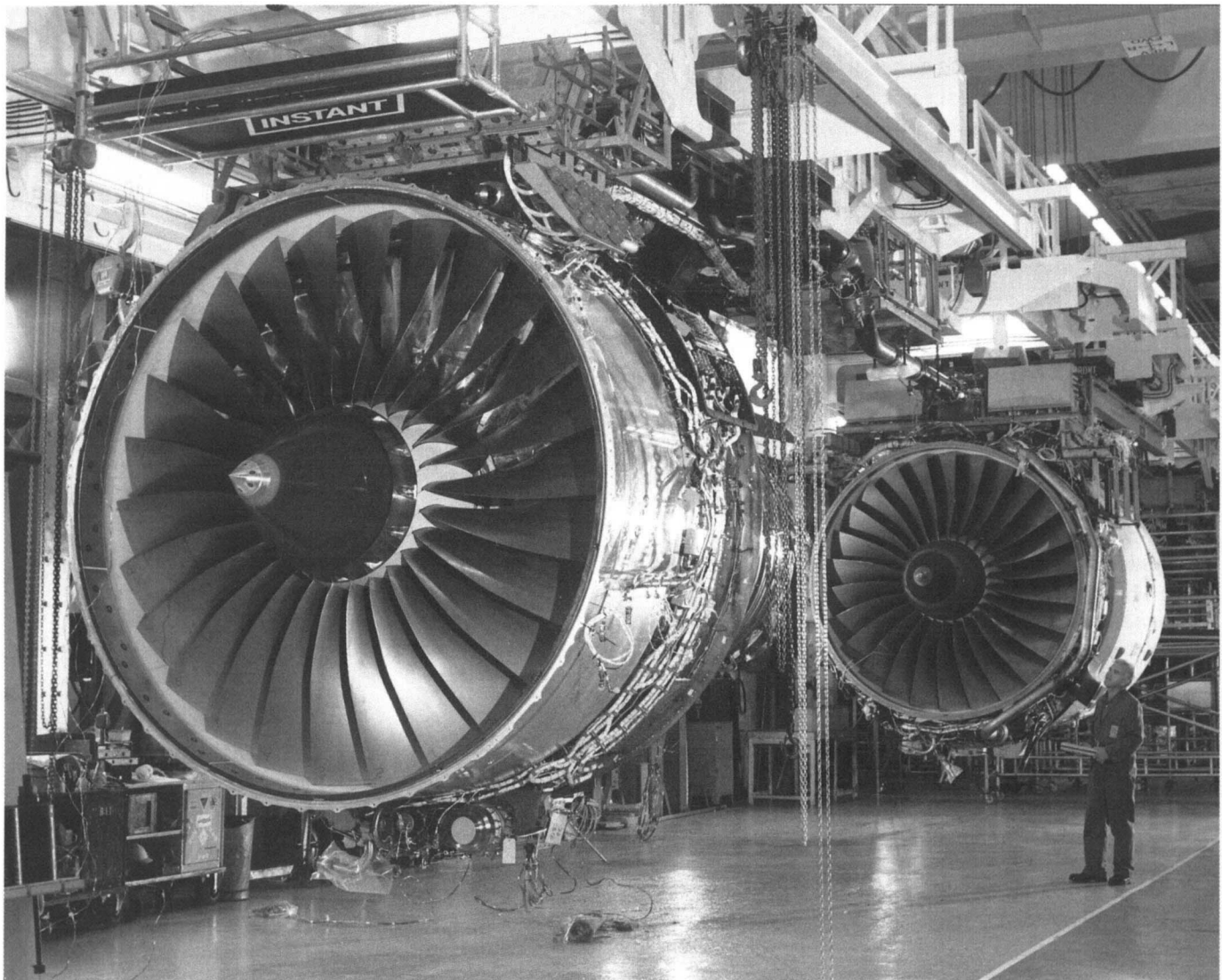
R Biggest of the Trents is the 800 family, much lighter than the competition yet with ratings up to 102,000 lb. In the background is a Trent 700, with a fan roughly a foot smaller in diameter.
