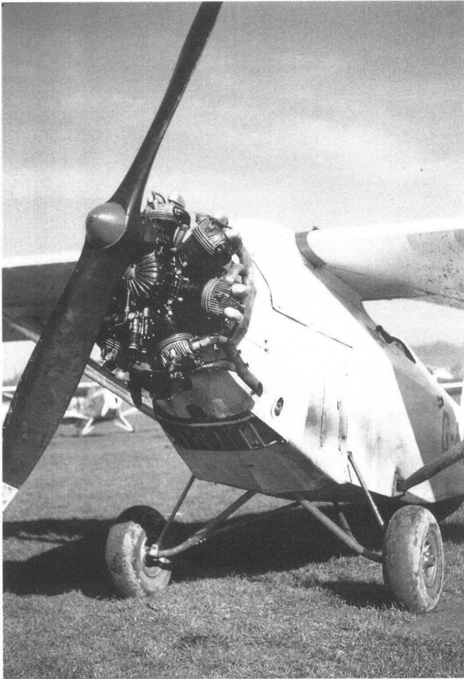
One of the first major applications for the Pobjoy R (Cataract) was the Comper Swift, made, like the engine, at Hooton Park, Cheshire. Extremely quiet, the engine was geared down to a big (78 in) propeller.
